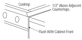
Front Flush With Cabinets - a Minimum of 25-3/4" Cabinet Depth Required
